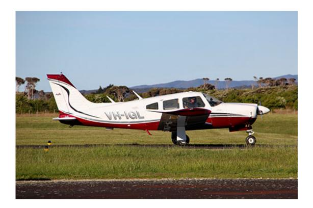
Aircraft Type: Piper Arrow PA28R Owners: Ian Tucker, Vicky Jiles Year: 1977 **Registration: VH-IGL** Number of Seats: 4 Engine: 200hp Fuel Injected Propeller: Constant Speed (Variable Pitch) Undercarriage: Retractable Normal Cruise Speed: 135 knots Max Speed 152 knots Stall Speed: 55 knots Rate of Climb 900 feet per minute Fuel Burn Rate: 45 litres/hour Fuel Capacity: 180 litres Endurance: 4 hours (approx 640 nautical miles) Empty Weight: 777 kg Maximum Take-Off Weight: 1205 kg
